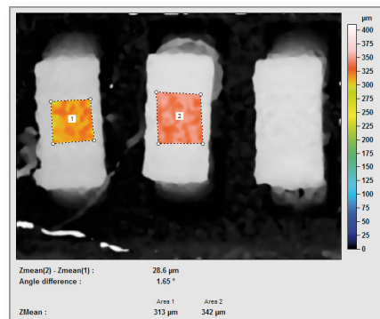
Coplanarity of contact zones on an electronic component using the step height (surfaces) study
