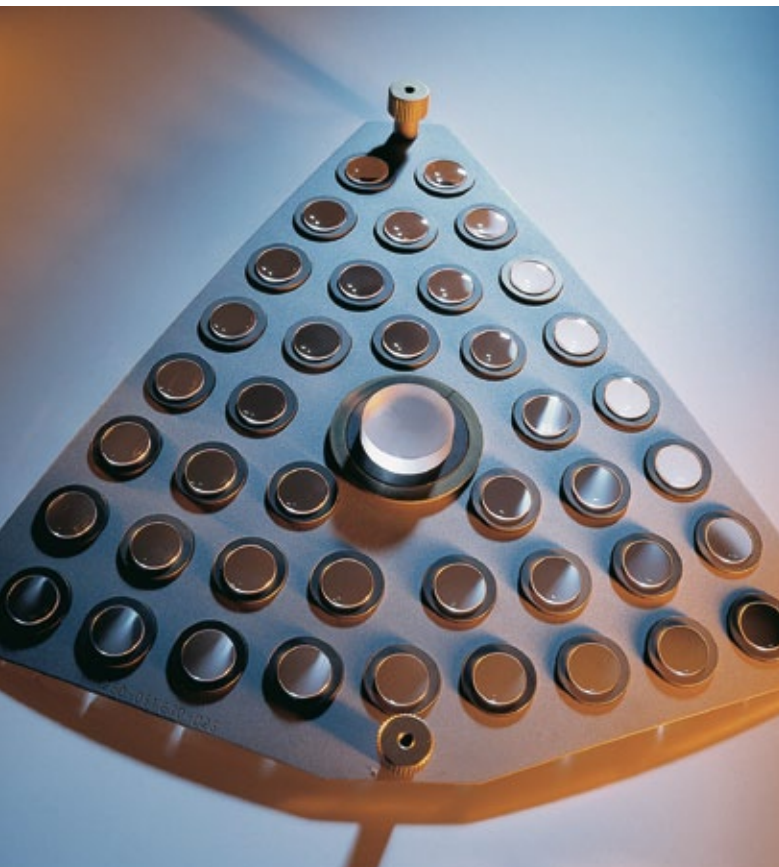
A selection of hand-polished lenses which form the core of our objectives
